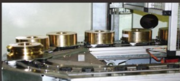
"Carrousel" reaching a capacity of 23 pieces up to 35 kg
