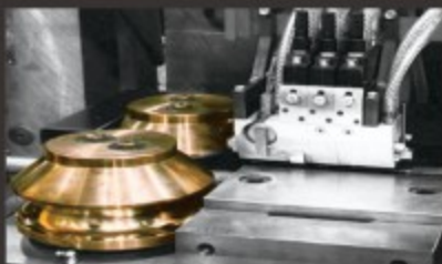
TIG process. Welding rolls and clamp guides in AMPCO® 21
