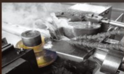
AMPCO® 25 rolls maintaining the tube during external deburring
