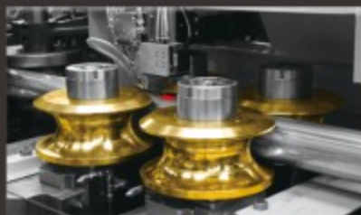
Laser process. Welding rolls in AMPCO® 25
