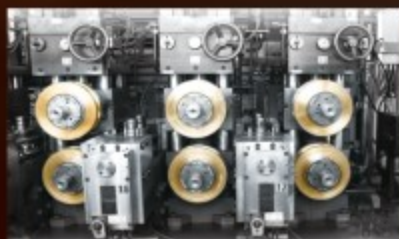
HF process. Sizing rolls in AMPCO® 25
