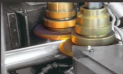
HF process. Welding rolls in AMPCO® 25
