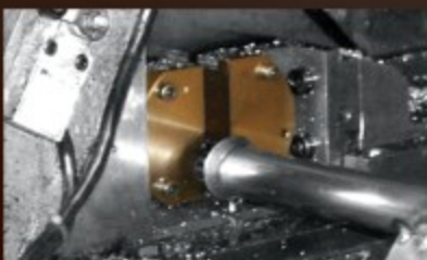
Laser process. Jaws in AMPCO® 18
