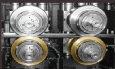
HF process. Forming rolls. Flanges in AMPCO® 25
