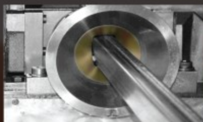
Saw guide in AMPCO® 18 for high strength hollow section
