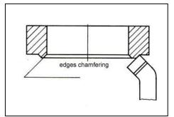
For roughing or finishing it is best to use hard metal cutting tool tips in the quality K10 / K20. For real fine machining (hole-shaft fits) a very good surface condition (N3) can be achieved with diamond tooling (PKD).
